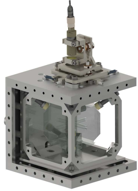
Fig. 4. Model of a 5 cm cube cavity mounted in a tetrahedral configuration with parts of the two-layer thermal shield. Attached to the top one is a 6-axis translation stage for direct in-coupling.
